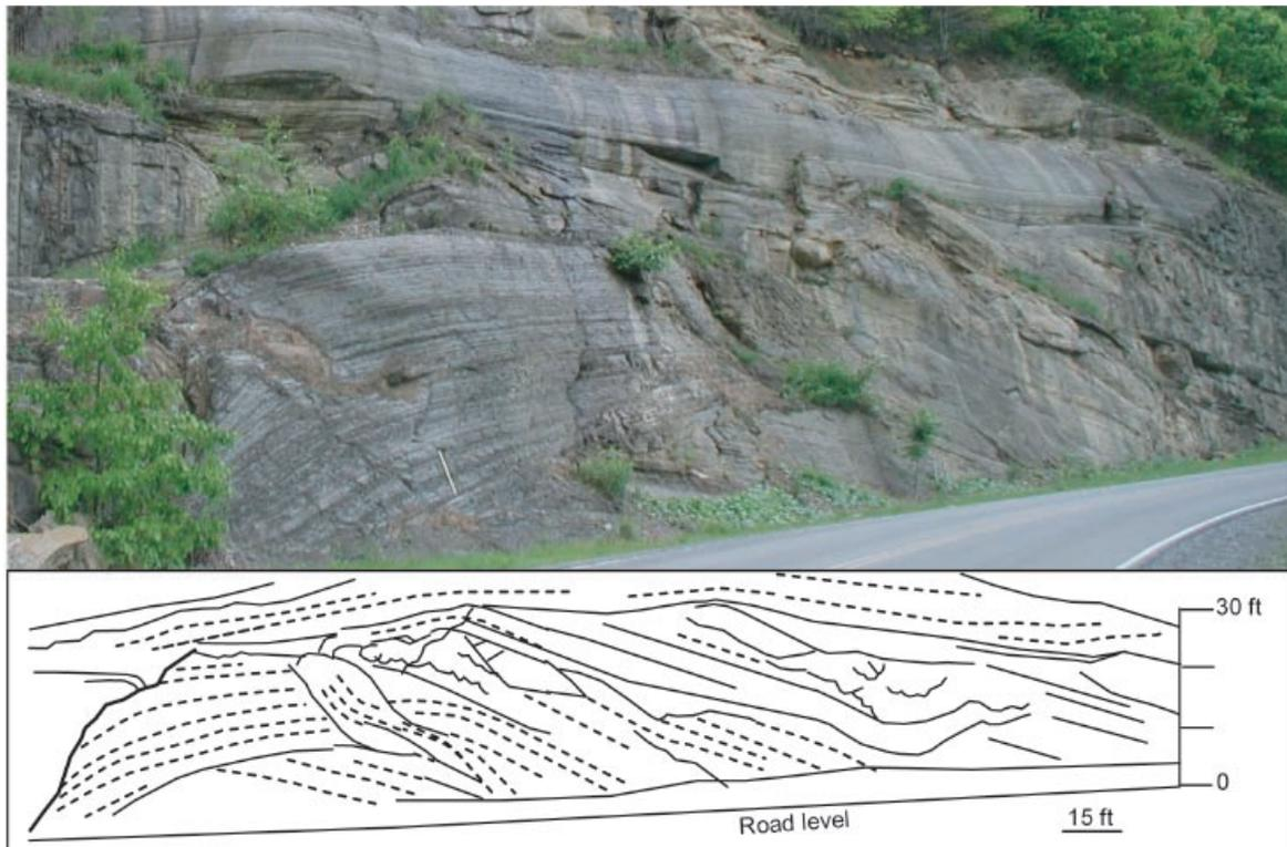
Figure 13. Large paleoslump (oblique view) in the Betsie Shale on Highway 609. Yardstick scale in photograph. The line drawing is a preliminary trace of a photomosaic (at right angles to the road) of the paleoslump, showing the numerous discontinuities within the slump block.
