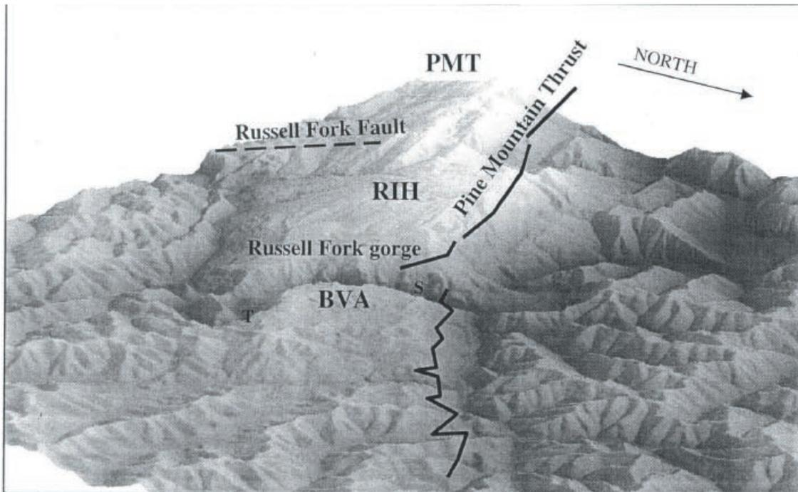
Figure 4. Oblique digital view of field trip area, showing three distinct topographic highs discussed in the text and the trace of faults discussed in the text. PMT: sharp linear ridge of Pine Mountain Thrust Sheet to the southwest; RIH: rotated beds of the intermediate high; BVA: anticline in the Breaks Interstate Park visitors area; S: Stateline Overlook; T: Towers Overlook.
